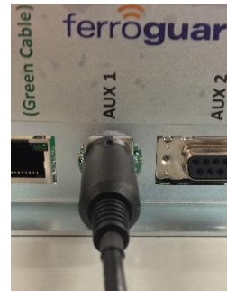
Figure 6 - Connection to AHUB.
