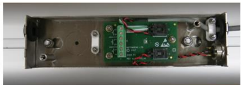
Secure brackets by tightening set screws, then fit & secure AOM by tightening locking nuts.
