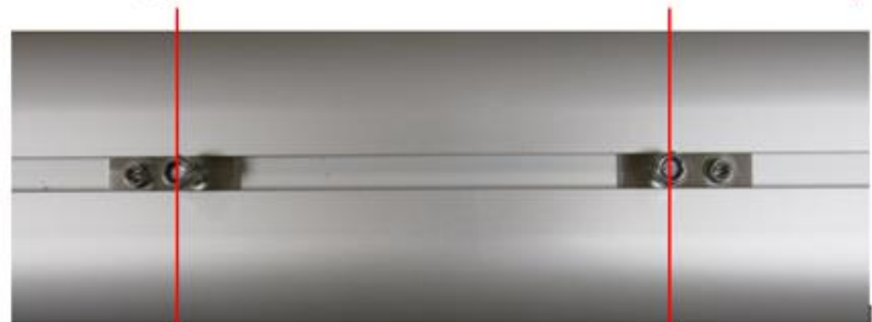
Measure from M6 stud centers to bottom of aluminum casing.
